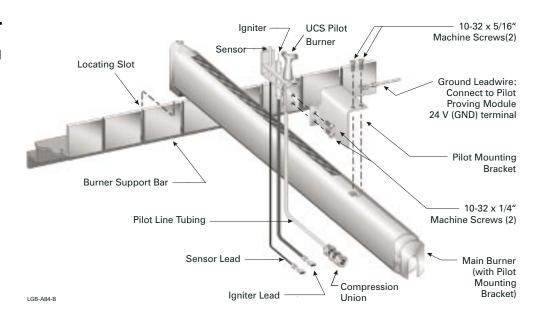
Figure 2 Main flame sensor assembly
